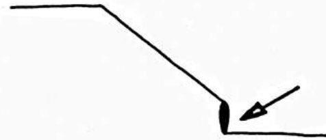
Undercutting of slope
