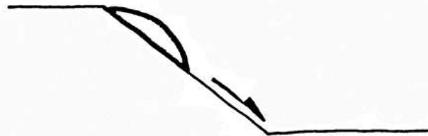
Addition of debris to slope
